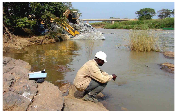
Figure 8B. Obtaining a surface water sample for turbidity analysis.
